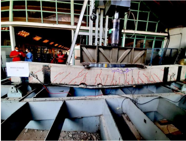
(a) Brittle failure in Specimen A1
