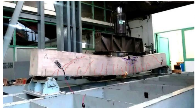
(a) Ductile failure in Specimen AN
