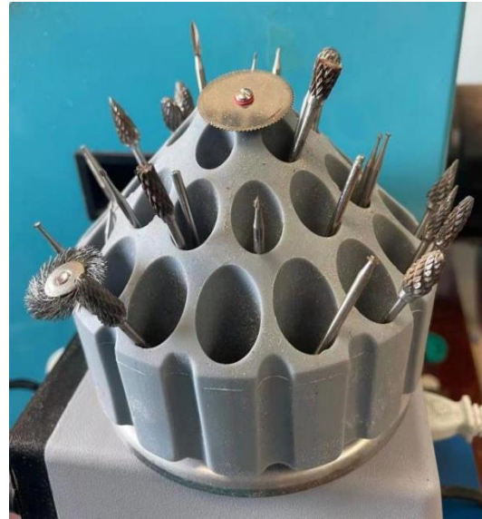
Fig. 5 Wood carving head of carving machine
