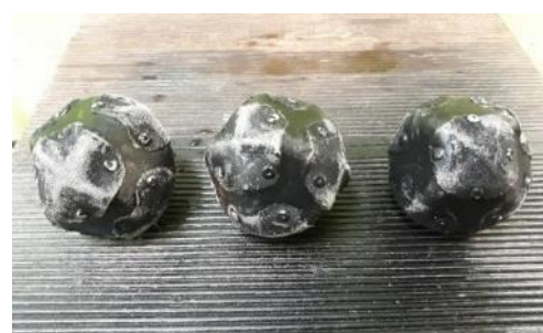
Fig. 4. Hollow balls as natural zeolite place.
