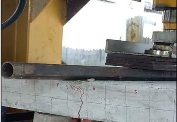
Fig. 9. Cracks formed in all flexure tested slabs.
