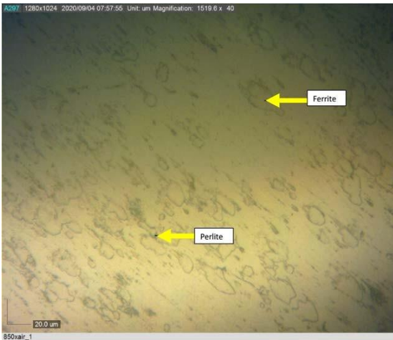
Fig. 6. The microstructure of the carburizing process at a temperature of 850 C with water quenching media for candlenut shell carbon charcoal.
