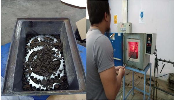
Fig. 2. Stages of the Carburizing Process.
