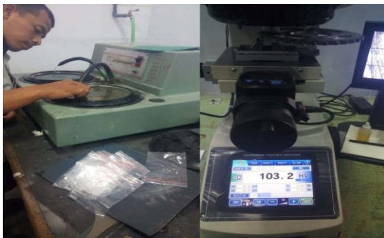
Fig. 4. Specimen polishing process and microstructure test.
