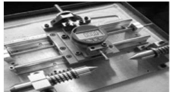
Fig. 7. Precision tapered workpiece measuring tool unit being calibrate for center alignment.
