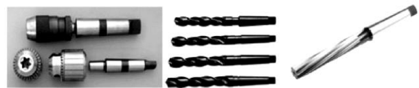
Fig. 1. Drill chucks, drill bits, and reamer having tapered shafts with a certain taper standard.
