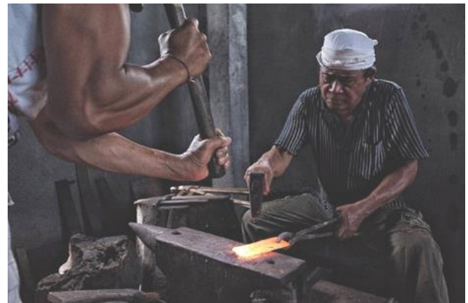
Fig. 2. Forging an iron with conventional tools.
