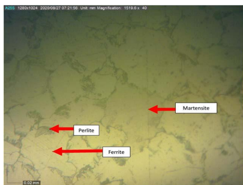
Fig. 9. Microstructure photo at 900°C with holding for 90 minutes.
