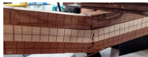
Figure 11 Type-A test object damage pattern (nail distance 10 cm).
