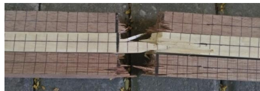
Figure 12 Type B test object damage pattern (nail distance 15 cm).
