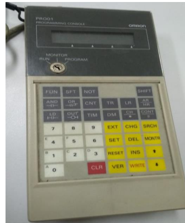
Figure 3. Console PLC C28H
