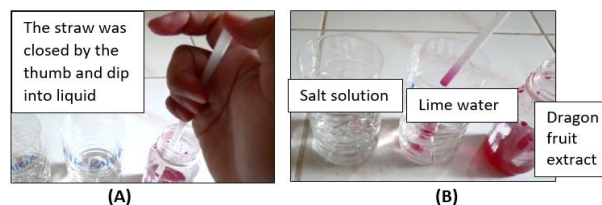
Figure 3 A simple procedure for taking materials using a straw as a feeding device instead of dropper pipette (A) fluid collection and (B) fluid drip.
