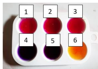
Figure 4 Observations of color changes in natural acid-base indicator practicum by using dragon fruit extract in several kind of solutions.
