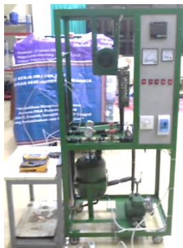
Figure 6 Oil cooler capacity test.
