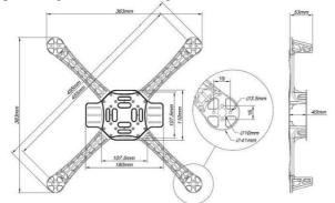
Figure 6. Dimensions of the quadcopter frame F450.
