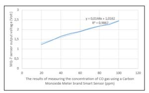
**Figure 5.** Graph of the relationship of CO gas concentration values measured using smart sensors with MQ-7 sensor output voltage.
