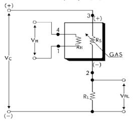
Figure 3. Schematic design of the MQ-7.
