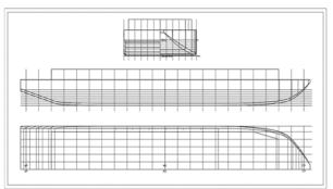
Figure 3. Lines Plan Floating Terminal.
