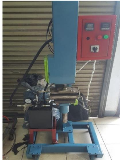
Figure 4. Plastic particle board press machine
