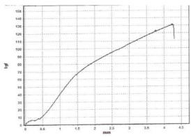
Figure 7. Tensile test results on HDU 8 Specimen
