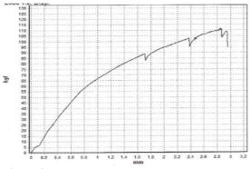
Figure 8. Tensile test results on HDU 12
