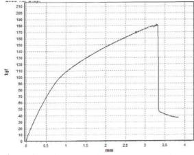
Figure 6. Tensile test results on HDU 4 . Specimen
