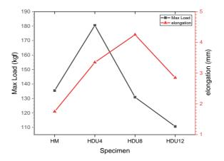
Figure 8. Tensile test results on HDU 12 Specimen
