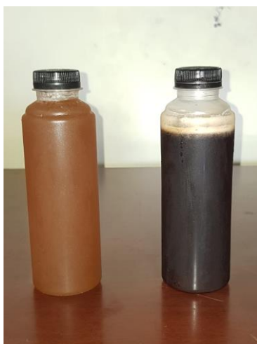
Figure 3. Physical comparison of sugar from vacuum evaporation (left) liquid sugar produced manually (right).
