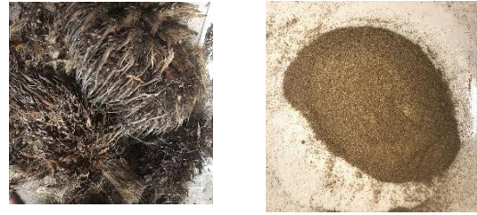
Figure 2 EFB (a) before size reducing and (b) after size reducing
