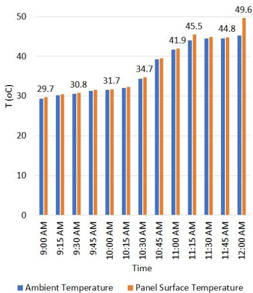
Figure 5 Ambient temperature and panel's surface temperature during the experiment
