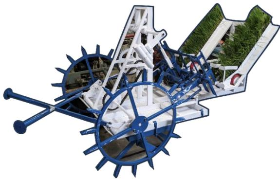
**Figure 4** Rice transplanter prototype for “tapak macan” cropping pattern
