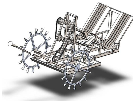
Figure 3 Design of rice transplanter prototype for “tapak macan” cropping pattern
