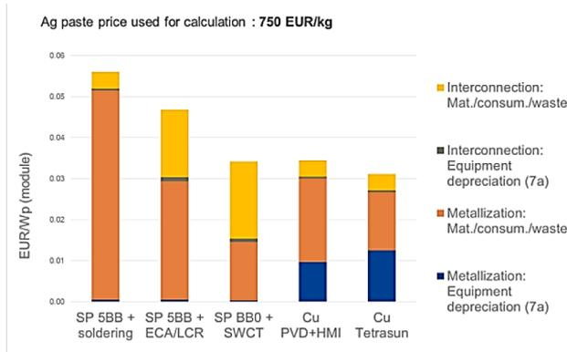
**Figure 1** Comparison of the outlay costs for the contact grid metallization.
