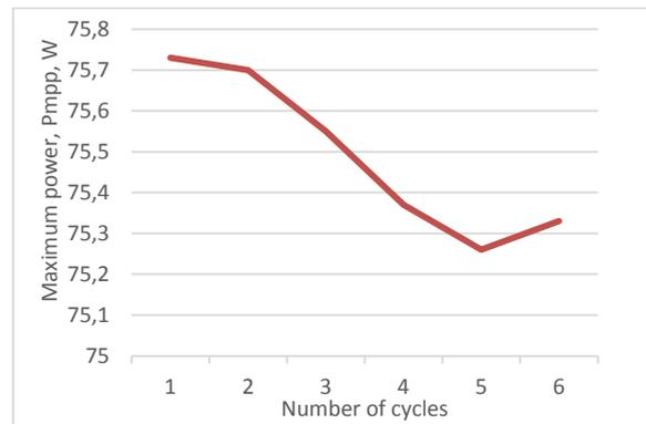
**Figure 6** Dependency graph of Pmpp solar module on the number of cycles passed in the climatic chamber, during thermal cycling test.
