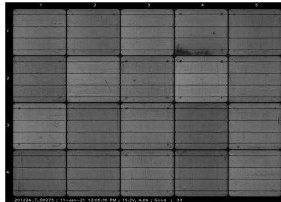
**Figure 8** Photoluminescence image of a solar module with copper contact grid solar cell after testing in a chamber of high humidity and temperature.
