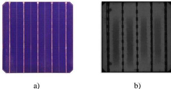
**Figure 3** Images of manufactured samples: a) frontal surface of solar cell; b) image of electroluminescence.
