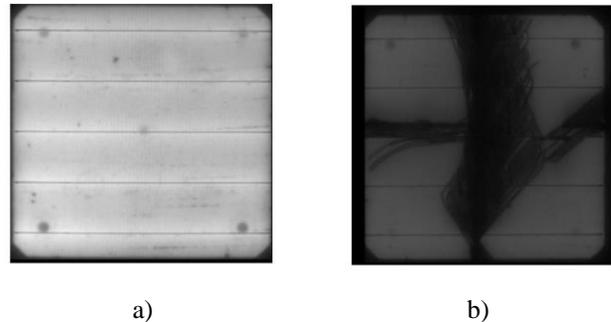
**Figure 4** Photoluminescence images of solar cells with a silver contact grid: a) before the mechanical impacts; b) after the mechanical impacts.
