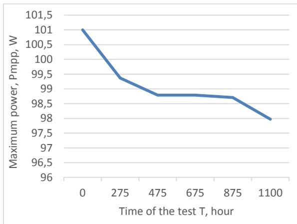
**Figure 7** Dependency graph of Pmpp solar module on the time in the climatic chamber when the damp heat test is passed.
