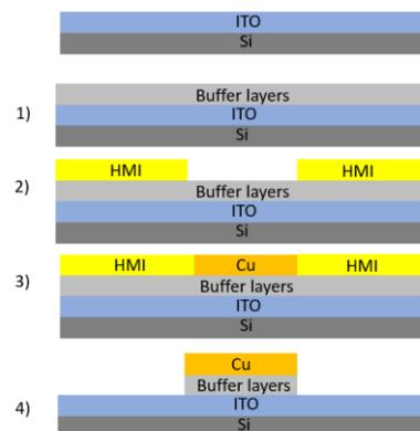
**Figure 2** Technological sequence of copper contour mesh forming.
