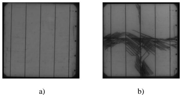
**Figure 5** Photoluminescence images of solar cells with a copper contact grid: a) before the mechanical impacts; b) after the mechanical impacts.
