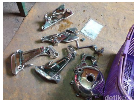
Fig. 3. Examples of chrome electroplating motorcycle accessories [3].
