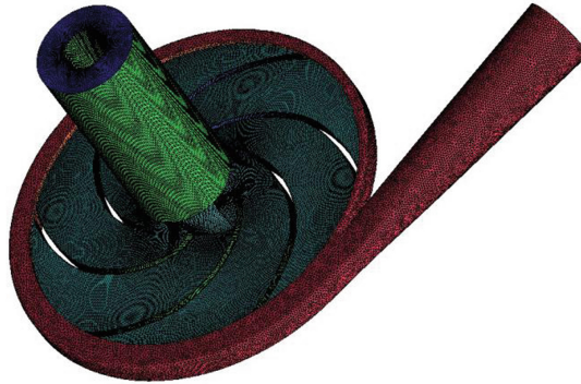
Fig. 2. Meshes of the centrifugal pump.
