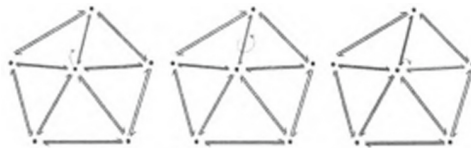
Fig. 2. One-ring field based on half-edge structure
