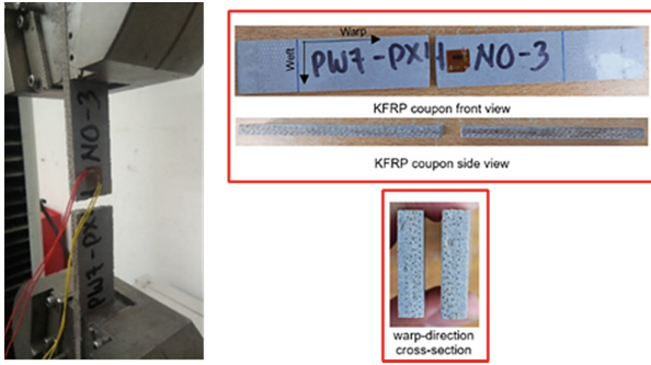
Fig. 5. Failure occurred within gauge length on KFRP unnotched coupon.
