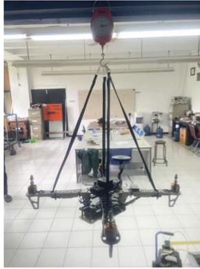
Fig. 1. Quadcopter Mass Measurement
