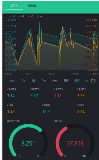
Fig. 3. Android app display of portable generator
