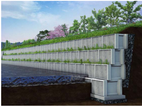
Figure 1 Schematic diagram of the industrial prefabricated bank revetment wall
