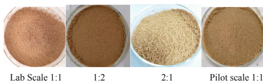
Fig. 1. Mengkudu spray dried powder from lab and pilot scale process
