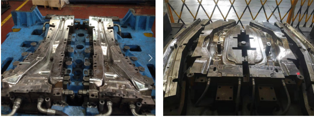
Fig. 3. Die of B-pillar and A-pillar lower panel.
