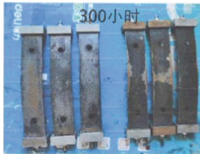
Fig. 14. Photos of bent over-yielding specimens soaked for 300 h.
