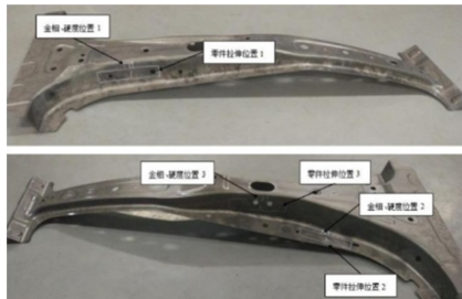
Fig. 3. Sampling and testing locations of the parts.
