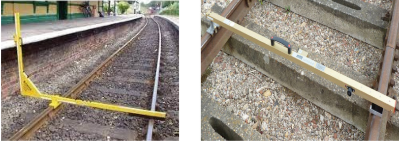
Fig. 1. Railroad Manual Measurement Tools: (a) Platform Gauge, (b) Meter Gauge
