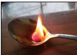
**Fig. 3.** Flame test of liquid smoke from HHW in this study.
