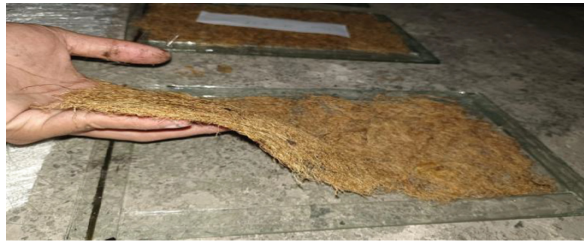
Fig. 2. Hand layup process
