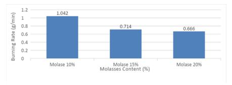
Fig. 1. Effect of Molasses Variations on Combustion Rate
