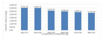
Fig. 5. Effect of Composition Comparison on Calorific Value
