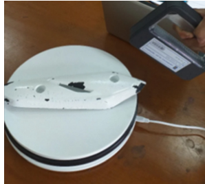
Fig. 5. Process of 3D Scanning
