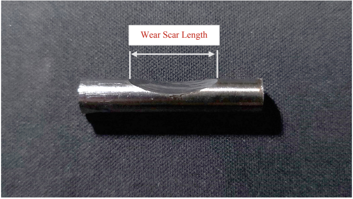
Fig. 4. Wear scar length of the wear test sample
