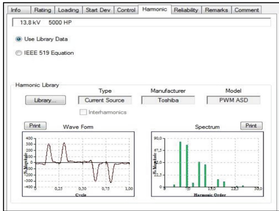
Fig. 4. The waveform and spectrum of harmonic source from ETAP
