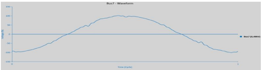
Fig. 11. Waveform of the bus 7 after installation of filters
