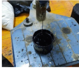
Fig. 11. Asphalt Penetration Test
