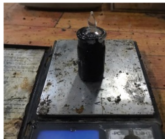
Fig. 10. Asphalt Specific Gravity Test
