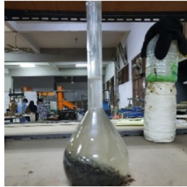
Fig. 8. Fine Aggregate Specific Gravity Test
