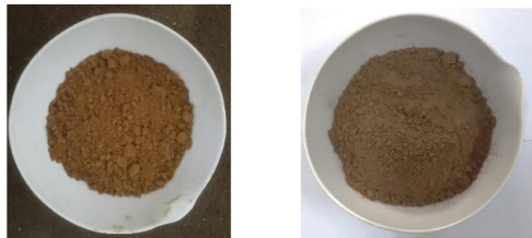
Fig. 2. Powdered Sample of (a) Palm Fiber, (b) Palm Leaves
