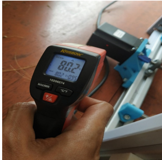
Fig. 3. Drive motor temperature check
