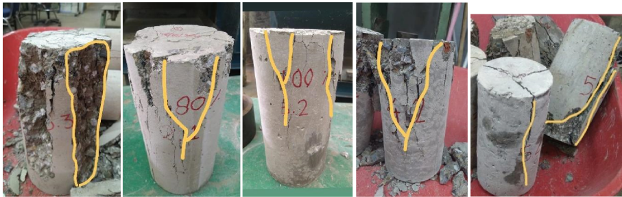
Fig. 3. Crack pattern of cylinder
