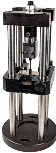
Fig. 4. Tensile test configuration.
