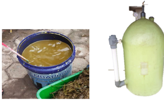
Fig. 1. Cow Manure and Fixed Dome Biogas Digester
