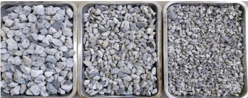
Fig. 3. The result of processing a concrete waste material from road construction
