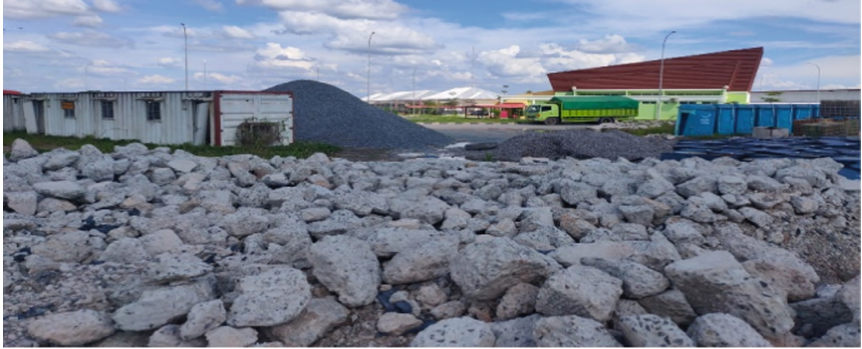
Fig. 1. Location where concrete waste materials from road construction was picked up
