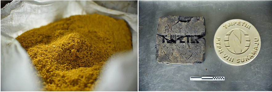
Fig. 10. Results of Gutta Percha Leaf Processing: Fine Jonjot (Yellow Solution) and White Gutta Slab, Past and Present (Source. Research Activities in Cipetir 2021. Modification of Lia Nuralia 2022)
