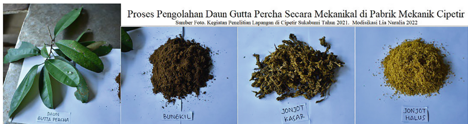
Fig. 9. Results of Processing of Gutta Percha Leaves at the Cipetir Mechanical Factory (Photo Source of Research Activities in Cipetir 2021. Modification by Lia Nuralia 2022)
