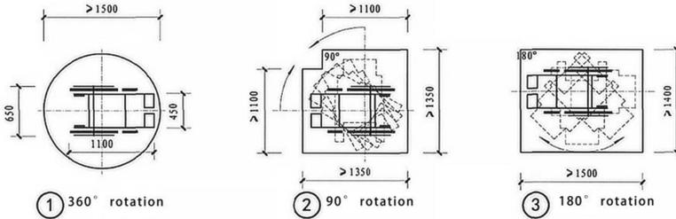
**Fig. 3.** Diagrammatic sketch of wheelchair rotation
