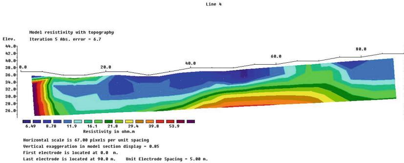
**Fig. 6.** Results of Wenner Geoelectric Processing 2D Track 4
