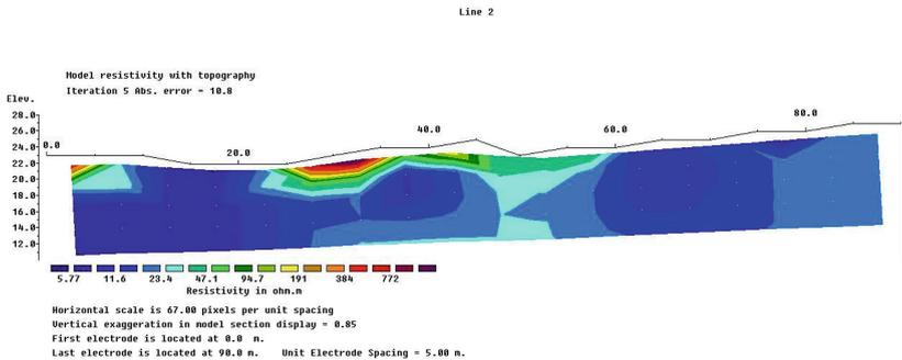
**Fig. 4.** Results of Wenner Geoelectric Processing 2D Track 2
