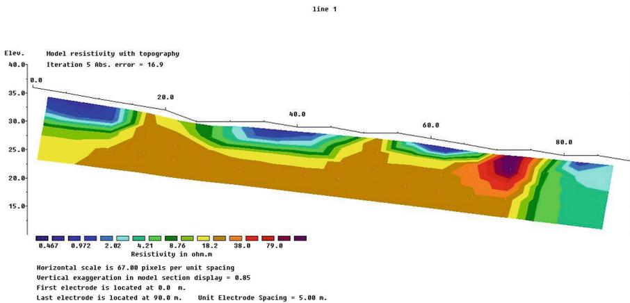
Fig. 3. Results of Wenner 2D Geoelectric Processing for Track 1
