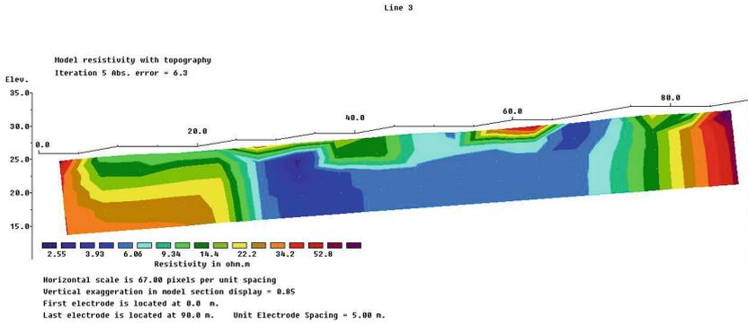
**Fig. 5.** The Result of Wenner 2D Geoelectric Processing for Track 3
