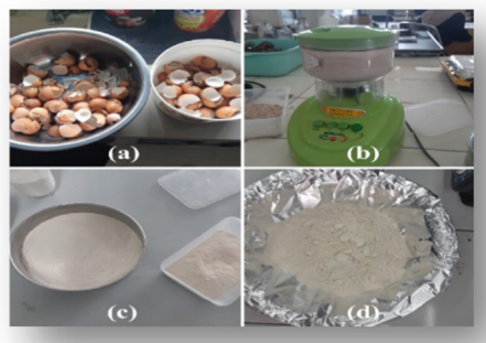
Fig. 1. The Preparation Process of Eggshell Powder as Adsorbent. (a) Eggshell Washing, (b) Reducing the Size of the Eggshell, (c) Sifting of Eggshell Powder, and (d) Eggshell Powder after Heating at 110 °C for 1 h
