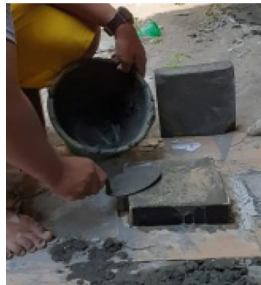
Fig. 3. Concrete moulding process.
