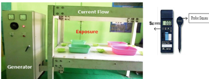
Fig. 2. ELF Electromagnetic Field Source Generator and EMF-meter
